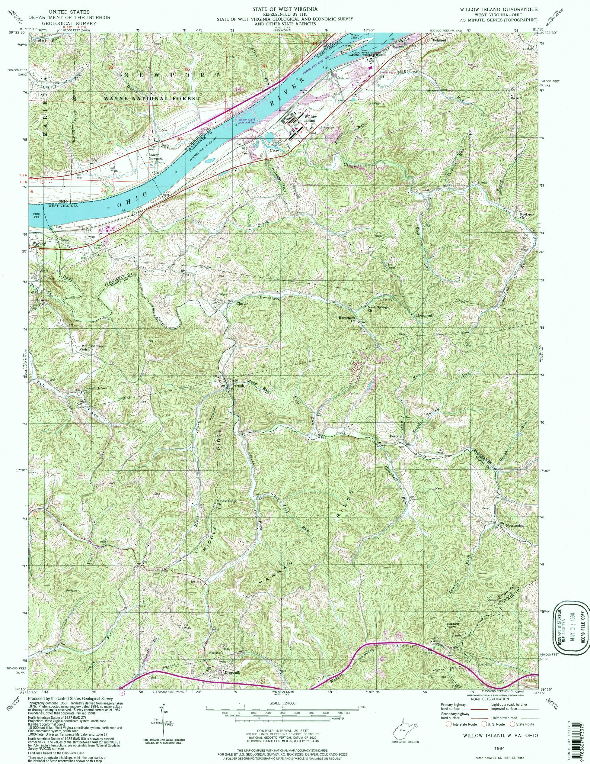
10 000-foot ticks: West Virginia coordinate system, north zone and Ohio coordinate system, south zone 1000-meter Universal Transverse Mercator grid, zone 17 North American Datum of 1983 (NAD 83) is shown by dashed corner ticks. The values of the shift between NAD 27 and NAD 83 for 7.5-minute intersections are obtainable from National Geodetic Survey NADCON software Land lines based on the Ohio River Base
