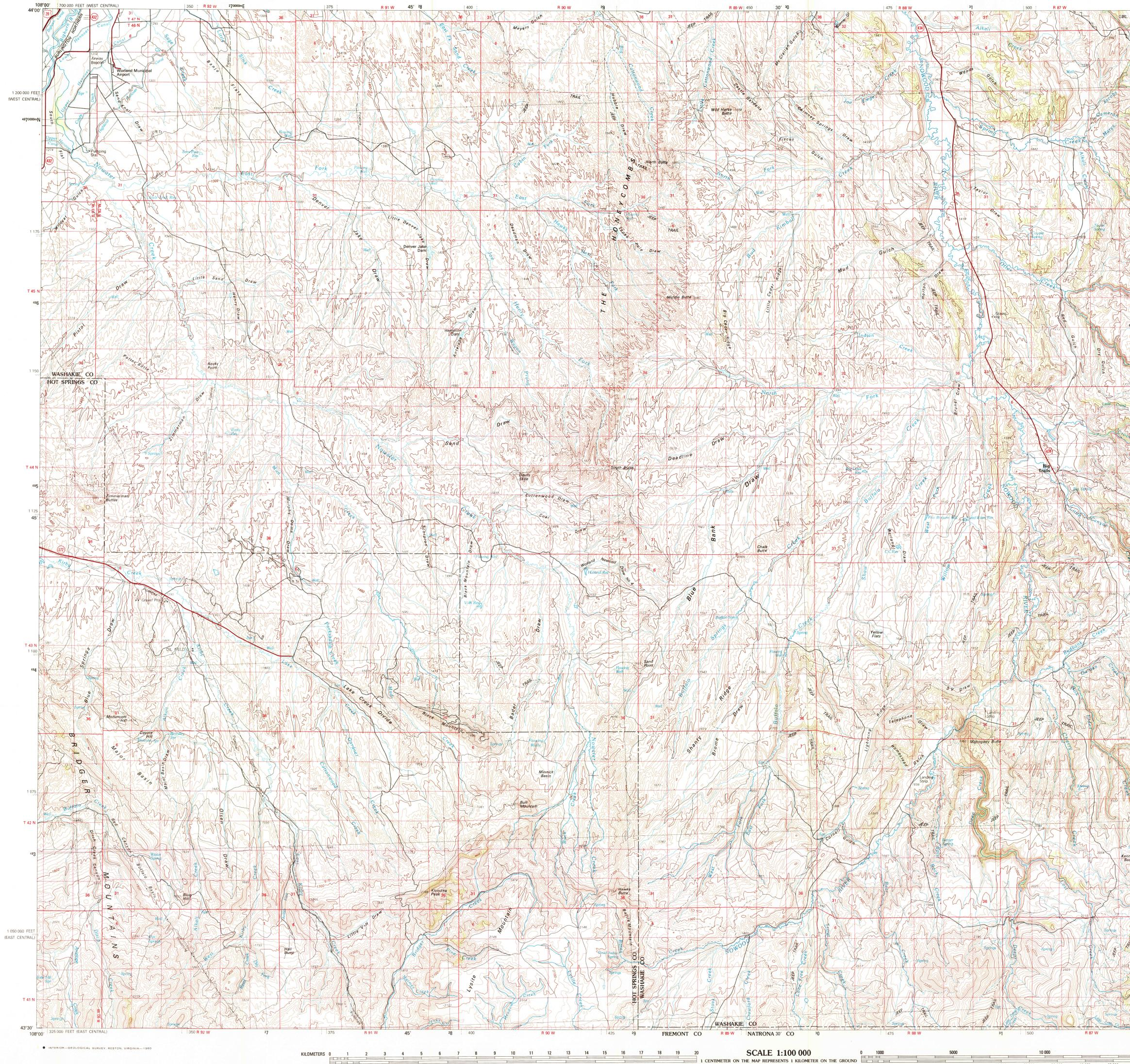
12 1 CENTIMETER ON THE MAP REPRESENTS 1 KILOMETER ON THE GROUND 12 CONTOUR INTERVAL 20 METERS
