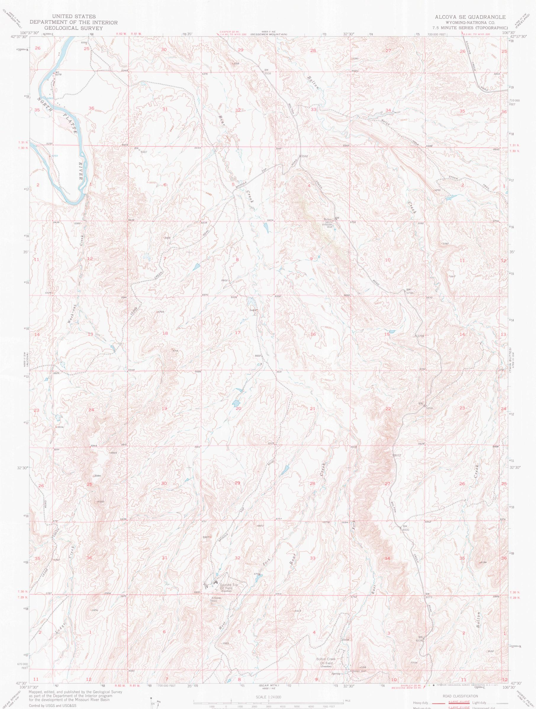
Control by USGS and USC&GS Topography from aerial photographs by multiplex methods Aerial photographs taken 1947. Field check 1950 Polyconic projection. 1927 North American datum 10,000-foot grid based on Wyoming coordinate system, east central zone
