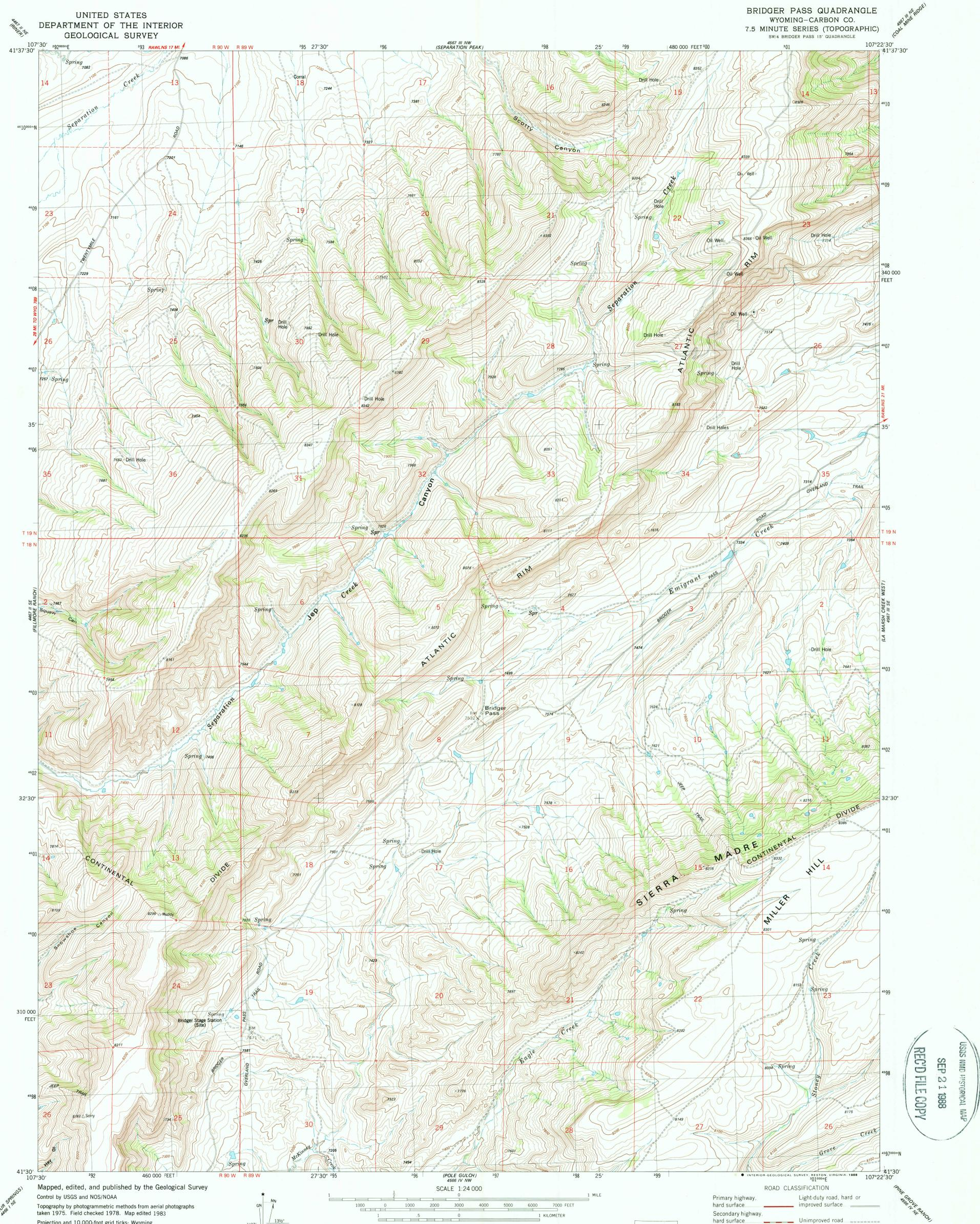
Projection and 10,000-foot grid ticks: Wyoming coordinate system, east central zone (transverse Mercator) 1000-meter Universal Transverse Mercator grid, zone 13 **1927** North American Datum To place on the predicted North American Datum 1983 move the projection lines 8 meters north and 52 meters east as shown by dashed corner ticks Fine red dashed lines indicate selected fence lines
