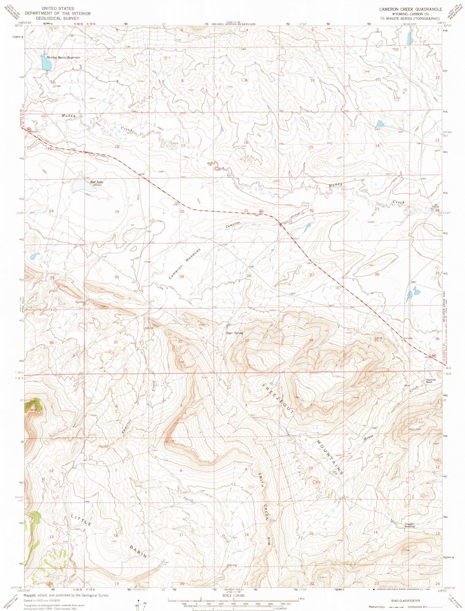
Polyconic projection. 1927 North American datum 10,000-foot grid based on Wyoming coordinate system. east central zone 1000-meter Universal Transverse Mercator grid ticks, zone 13, shown in blue
