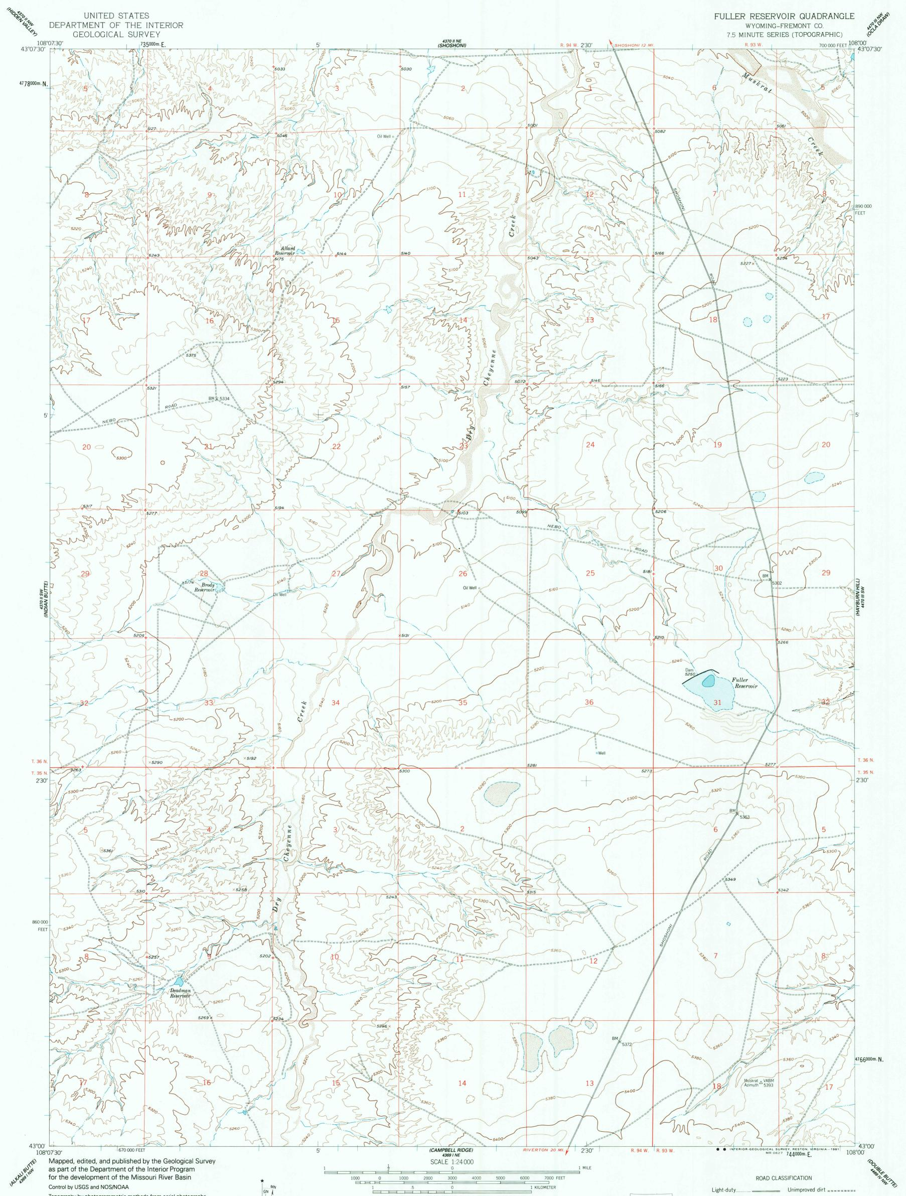
Topography by photogrammetric methods from aerial photographs taken 1949 and planetable surveys 1951. Revised 1960
