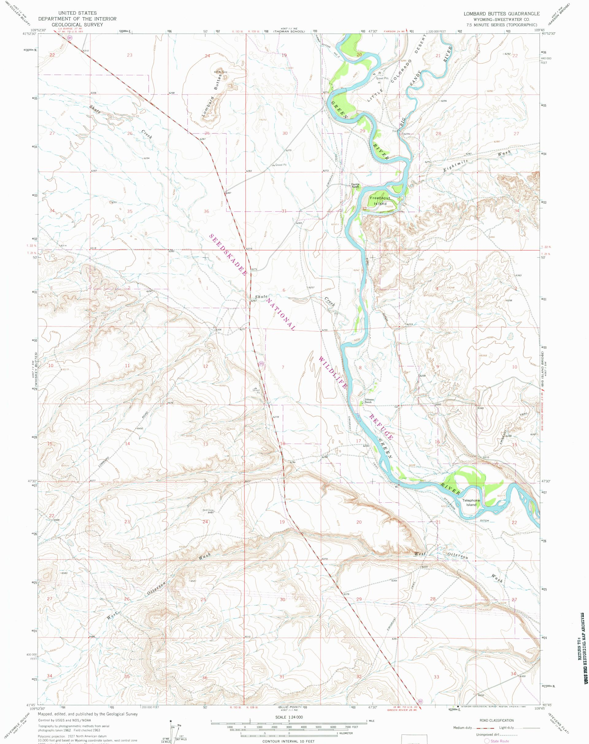
10,000-foot grid based on Wyoming coordinate system, west central zone 1000-meter Universal Transverse Mercator grid ticks, zone 12, shown in blue
