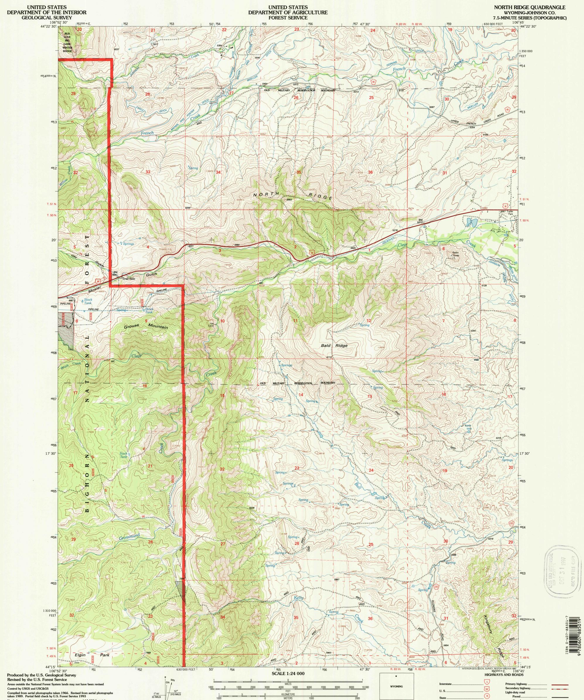
North American Datum of 1927 (NAD 27). Projection and 10 000-foot ticks: Wyoming coordinate system, east central zone (Lambert conformal conic). Blue 1000-meter Universal Transverse Mercator ticks, zone 13
