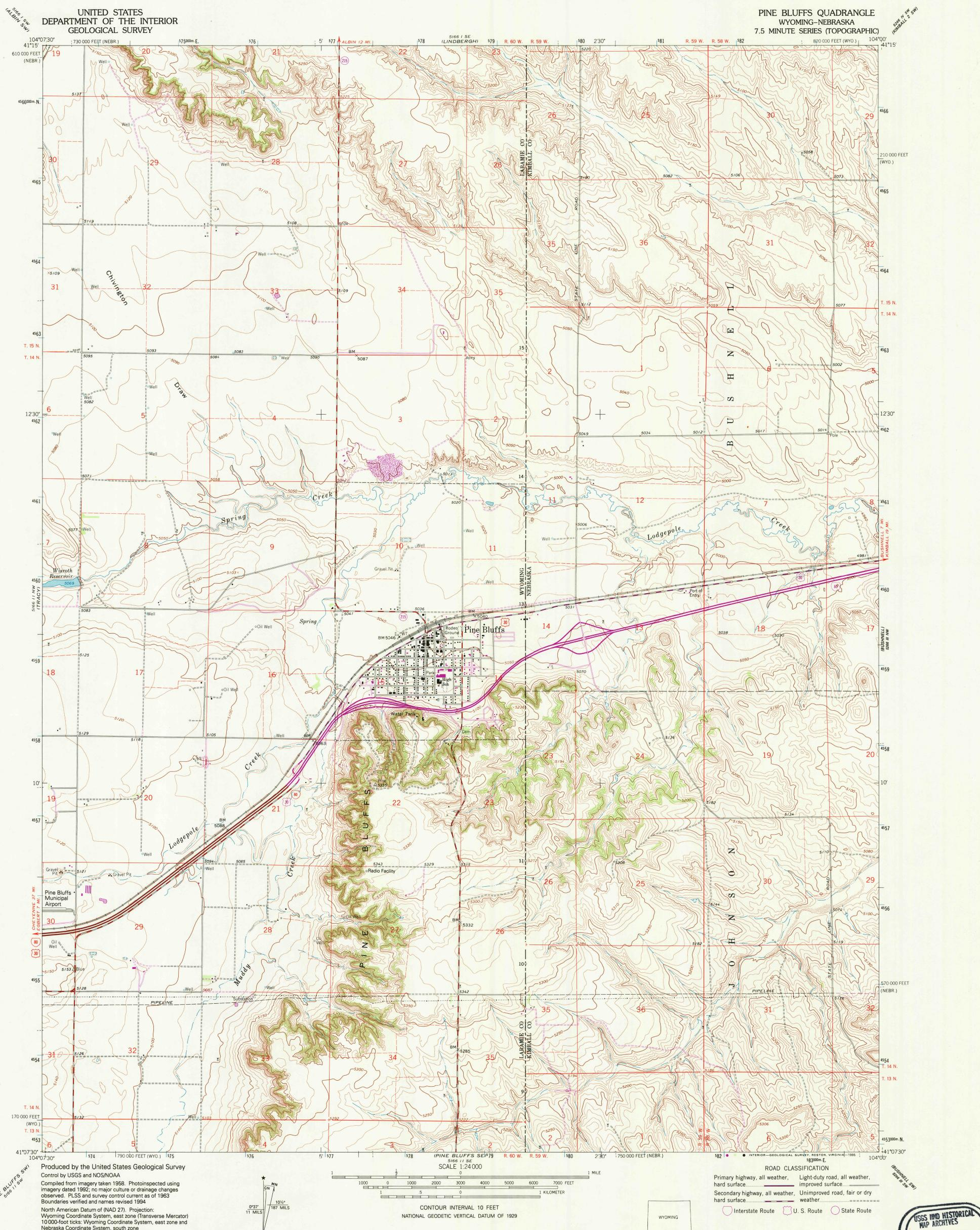
North American Datum of (NAD 27). Projection: Wyoming Coordinate System, east zone (Transverse Mercator) 10 000-foot ticks: Wyoming Coordinate System, east zone and Nebraska Coordinate System, south zone Blue 1000-meter Universal Transverse Mercator ticks, zone 13 North American Datum of 1983 (NAD 83) is shown by dashed. corner ticks. The values of the shift between NAD 27 and NAD 83 for 7.5-minute intersections are obtainable from National Geodetic Survey NADCON software
