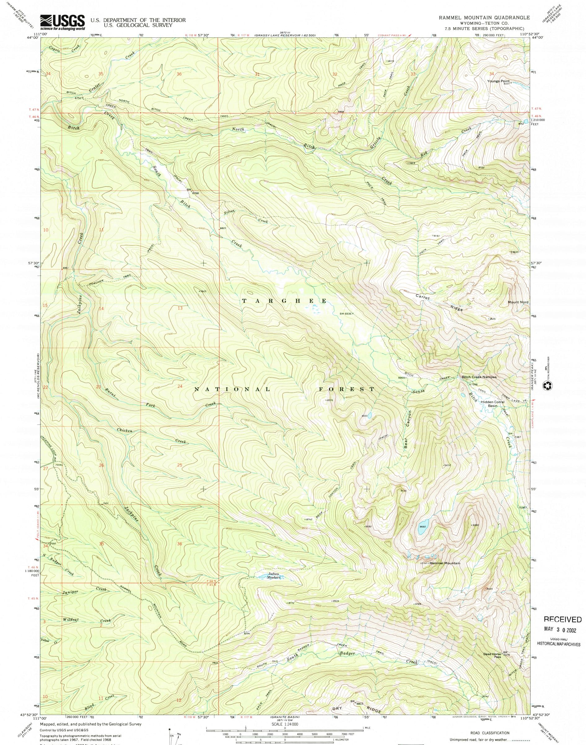
Polyconic projection. 1927 North American datum 10,000-foot grid based on Wyoming coordinate system, west zone 1000-meter Universal Transverse Mercator grid ticks, zone 12, shown in blue
