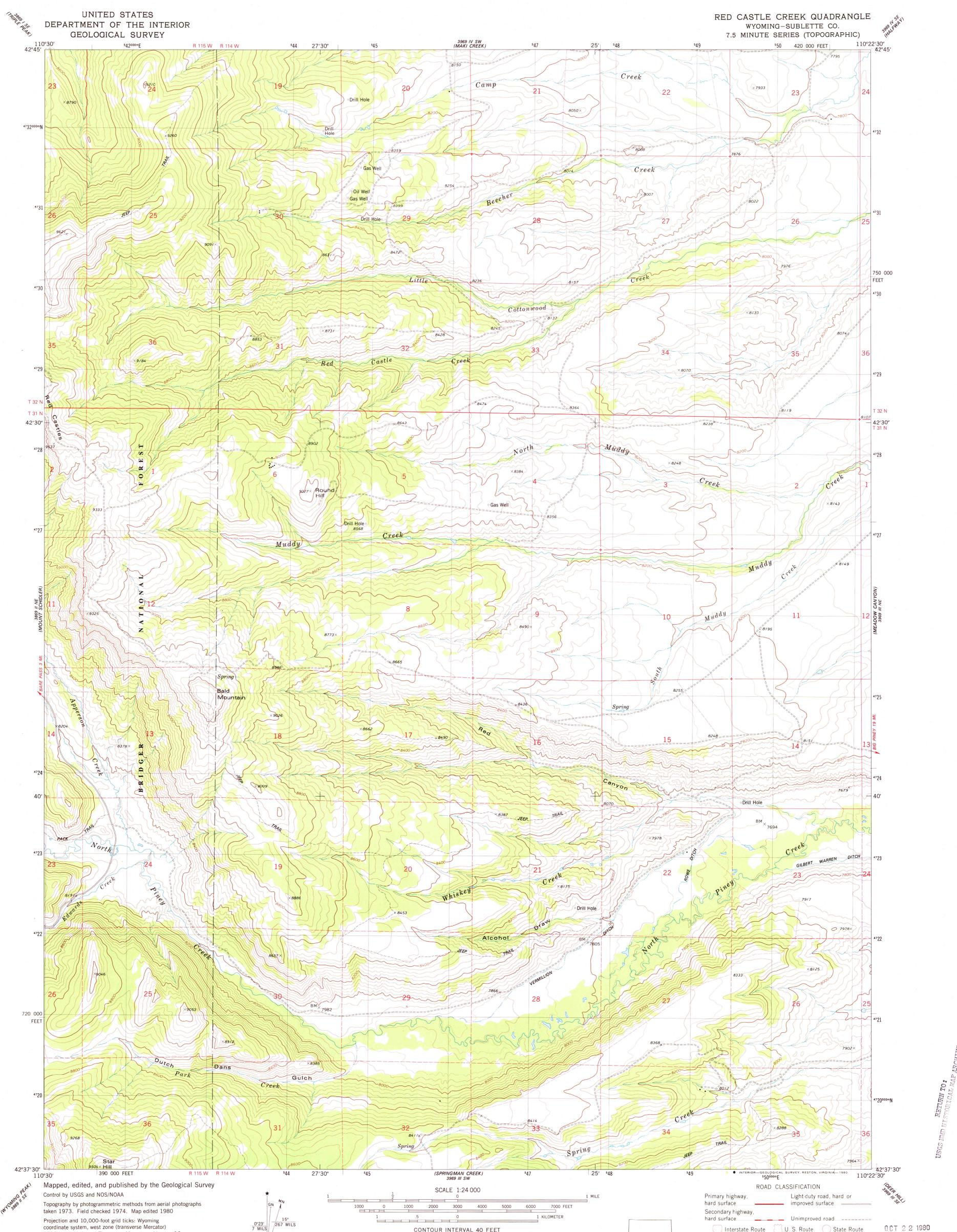
Projection and 10,000-foot grid ticks: Wyoming coordinate system, west zone (transverse Mercator) 1000-meter Universal Transverse Mercator grid, zone 12 1927 North American datum To place on the predicted North American Datum 1983 move the projection lines 11 meters north and 61 meters east as shown by dashed corner ticks Fine red dashed lines indicate selected fence lines There may be private inholdings within the boundaries of the National or State reservations shown on this map
