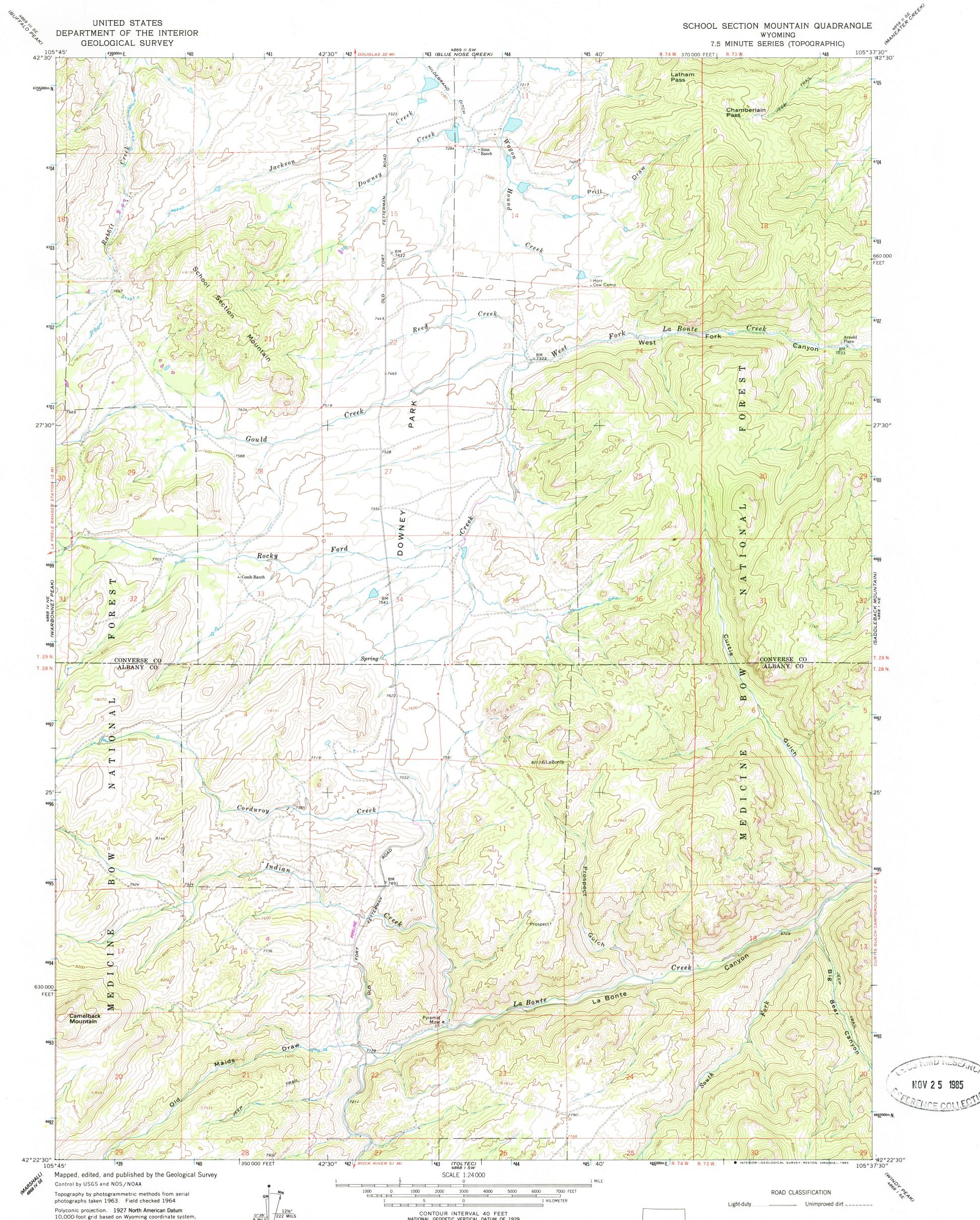
Polyconic projection. 1927 North American Datum 10,000-foot grid based on Wyoming coordinate system, east zone 1000-meter Universal Transverse Mercator grid ticks, zone 13, shown in blue Fine red dashed lines indicate selected fence lines To place on the predicted North American Datum 1983 move the projection lines 7 meters north and 48 meters east as shown by dashed corner ticks There may be private inholdings within the boundaries of the National or State reservations shown on this map
