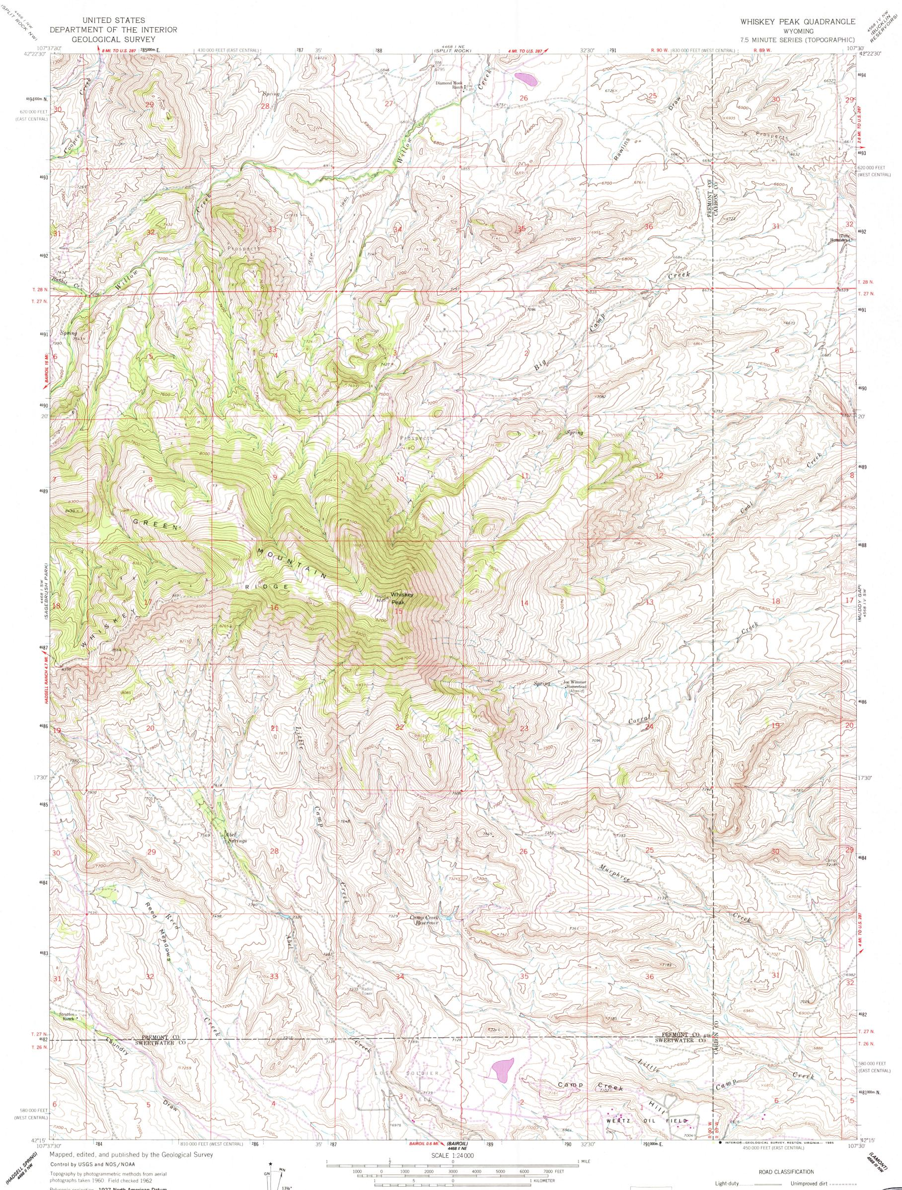
Polyconic projection. **1927 North American Datum** 10,000-foot grid based on Wyoming coordinate system, west central and east central zones 1000-meter Universal Transverse Mercator grid ticks, zone 13, shown in blue Fine red dashed lines indicate selected fence lines
