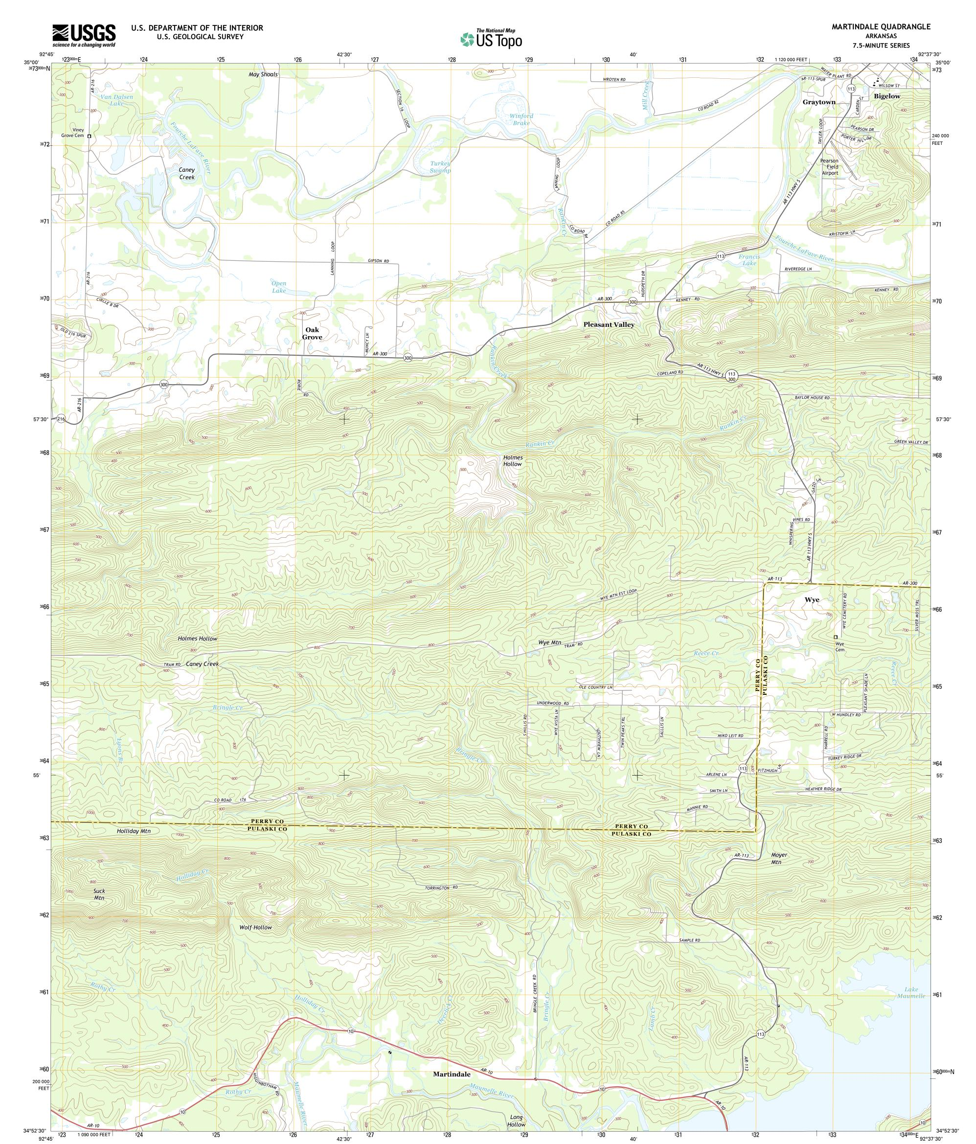
Produced by the United States Geological Survey North American Datum of 1983 (NAD83) World Geodetic System of 1984 (WGS84). Projection and 1 000-meter grid: Universal Transverse Mercator, Zone 15S 10 000-foot ticks: Arkansas Coordinate System of 1983 (north zone)
