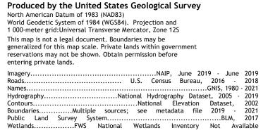
North American Datum of 1983 (NAD83) World Geodetic System of 1984 (WGS84). Projection and 1 000-meter grid:Universal Transverse Mercator, Zone 12S
