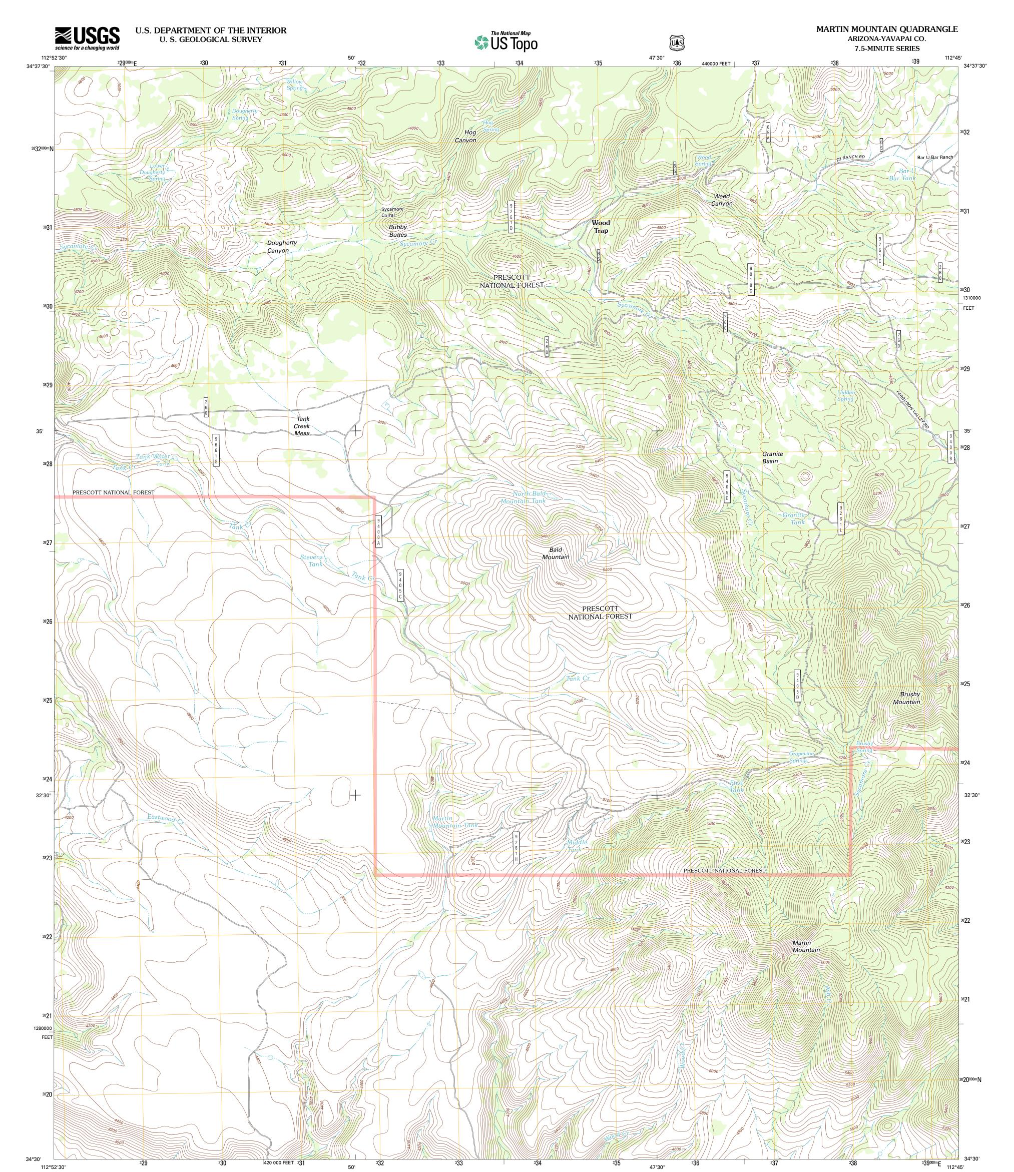
Produced by the United States Geological Survey North American Datum of 1983 (NAD83) World Geodetic System of 1984 (WGS84). Projection and 1 000-meter grid: Universal Transverse Mercator, Zone 12S 10 000-foot ticks: Arizona Coordinate System of 1983 (central zone)
