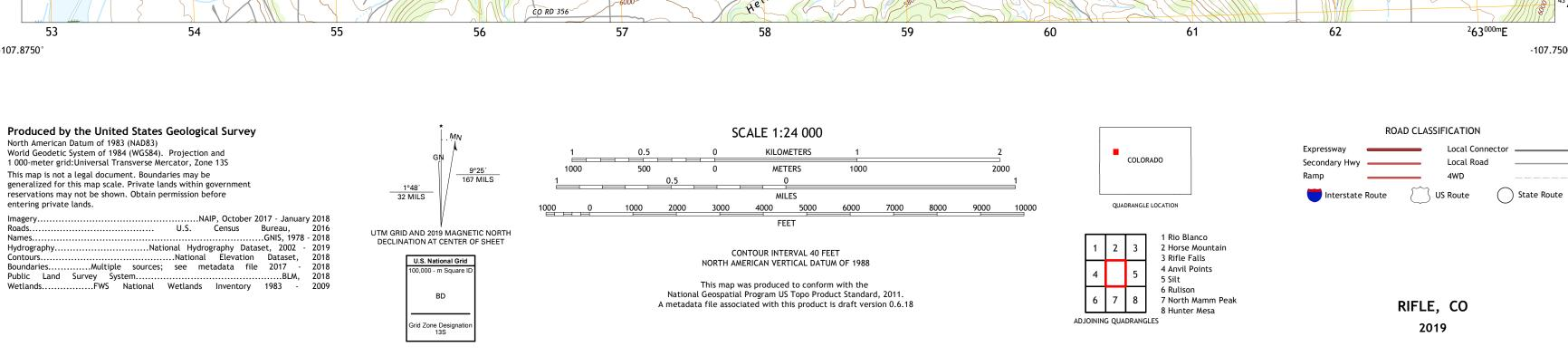
North American Datum of 1983 (NAD83) World Geodetic System of 1984 (WGS84). Projection and 1 000-meter grid:Universal Transverse Mercator, Zone 13S
