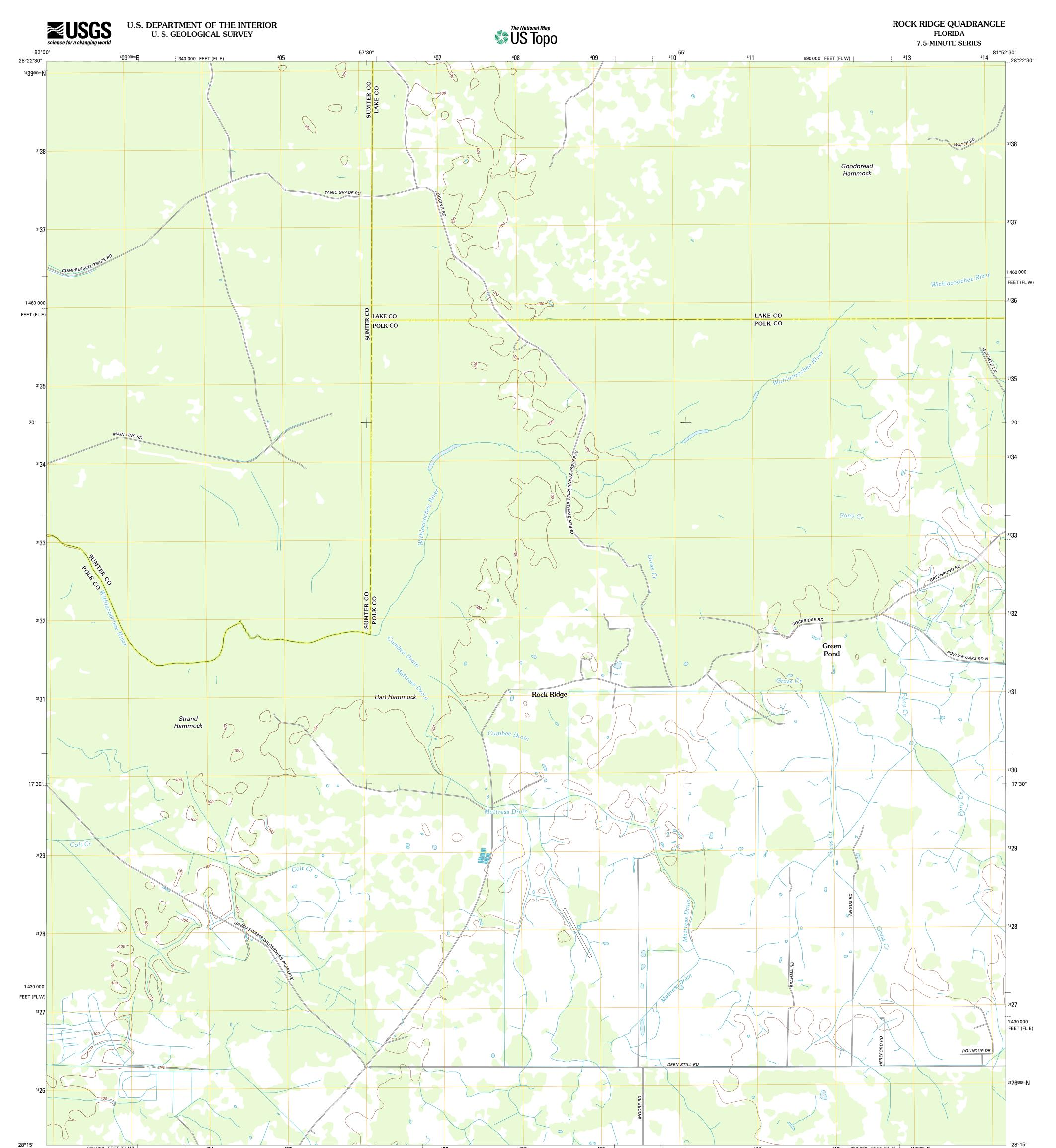
Produced by the United States Geological Survey North American Datum of 1983 (NAD83) World Geodetic System of 1984 (WGS84). Projection and 1 000-meter grid: Universal Transverse Mercator, Zone 17R 10 000-foot ticks: Florida Coordinate System of 1983 (west and east appead and east zones)
