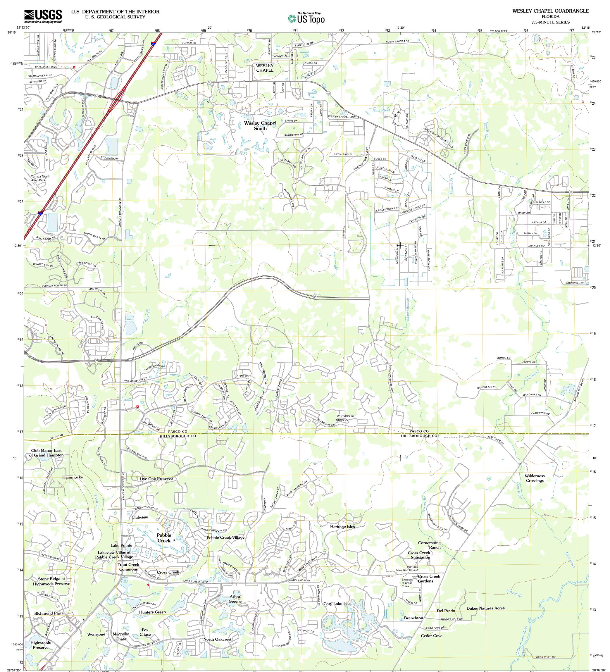
Produced by the United States Geological Survey North American Datum of 1983 (NAD83) World Geodetic System of 1984 (WGS84). Projection and 1 000-meter grid: Universal Transverse Mercator, Zone 17R 10 000-foot ticks: Florida Coordinate System of 1983 (west zone) zone)
