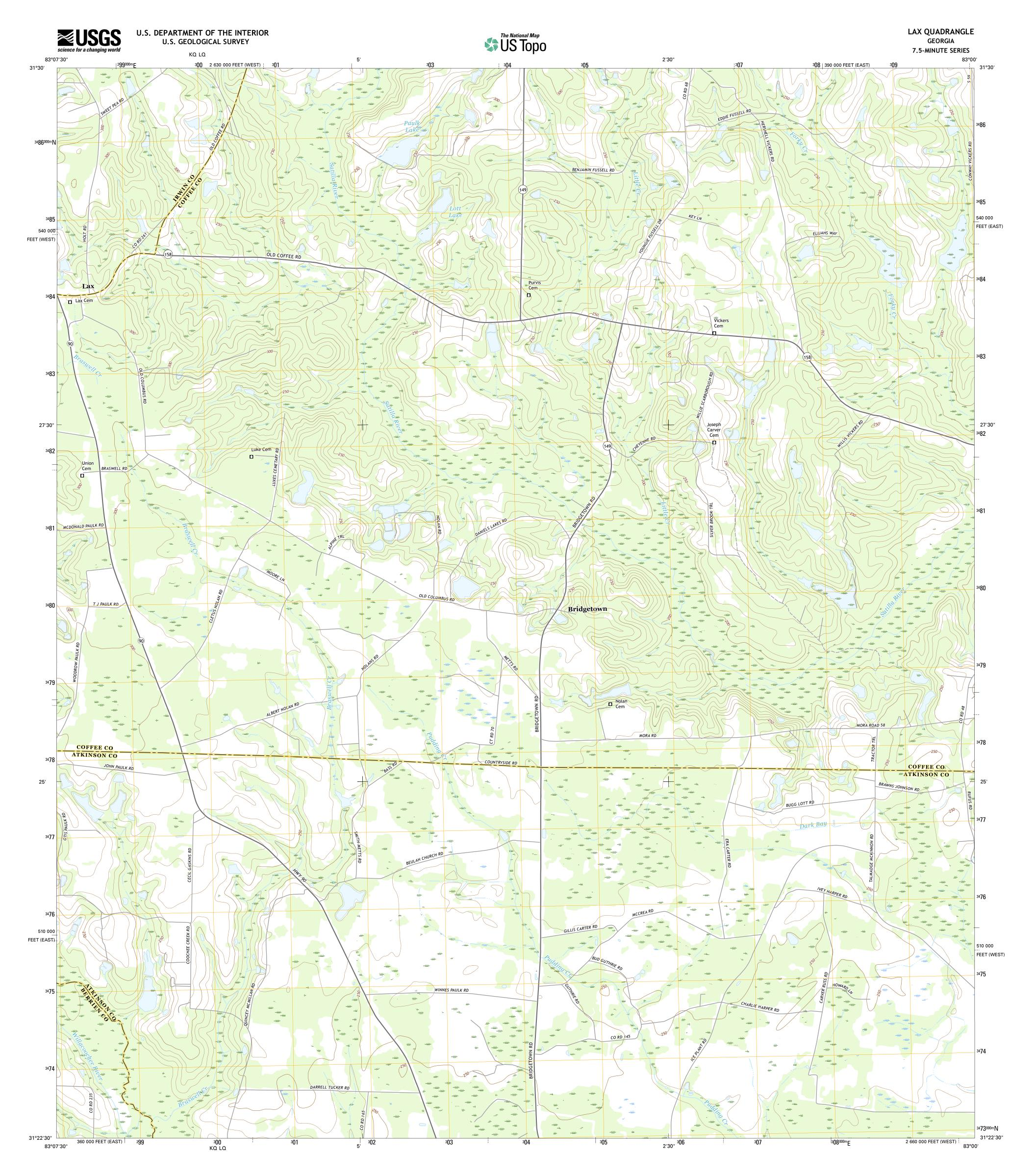
Produced by the United States Geological Survey North American Datum of 1983 (NAD83) World Geodetic System of 1984 (WGS84). Projection and 1 000-meter grid: Universal Transverse Mercator, Zone 17R 10 000-foot ticks: Georgia Coordinate System of 1983 (east and west zones)
