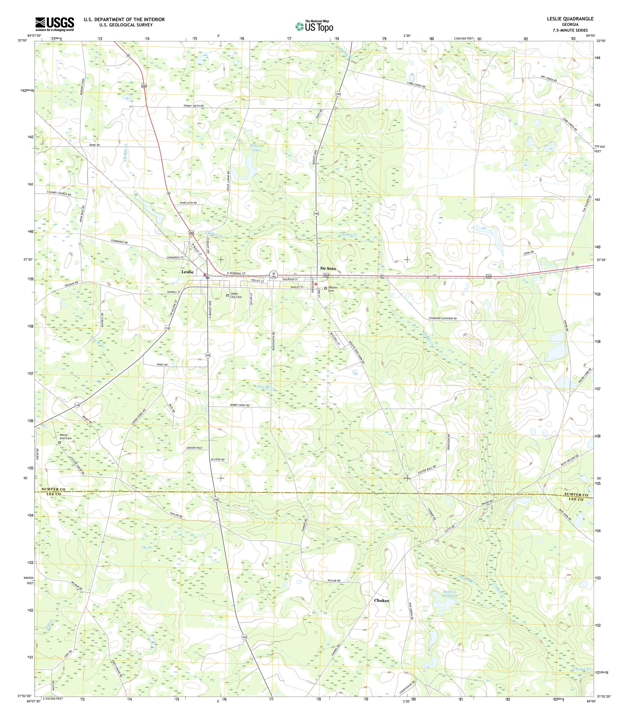
Produced by the United States Geological Survey North American Datum of 1983 (NAD83) World Geodetic System of 1984 (WGS84). Projection and 1 000-meter grid: Universal Transverse Mercator, Zone 16R 10 000-foot ticks: Georgia Coordinate System of 1983 (west Zone) zone)
