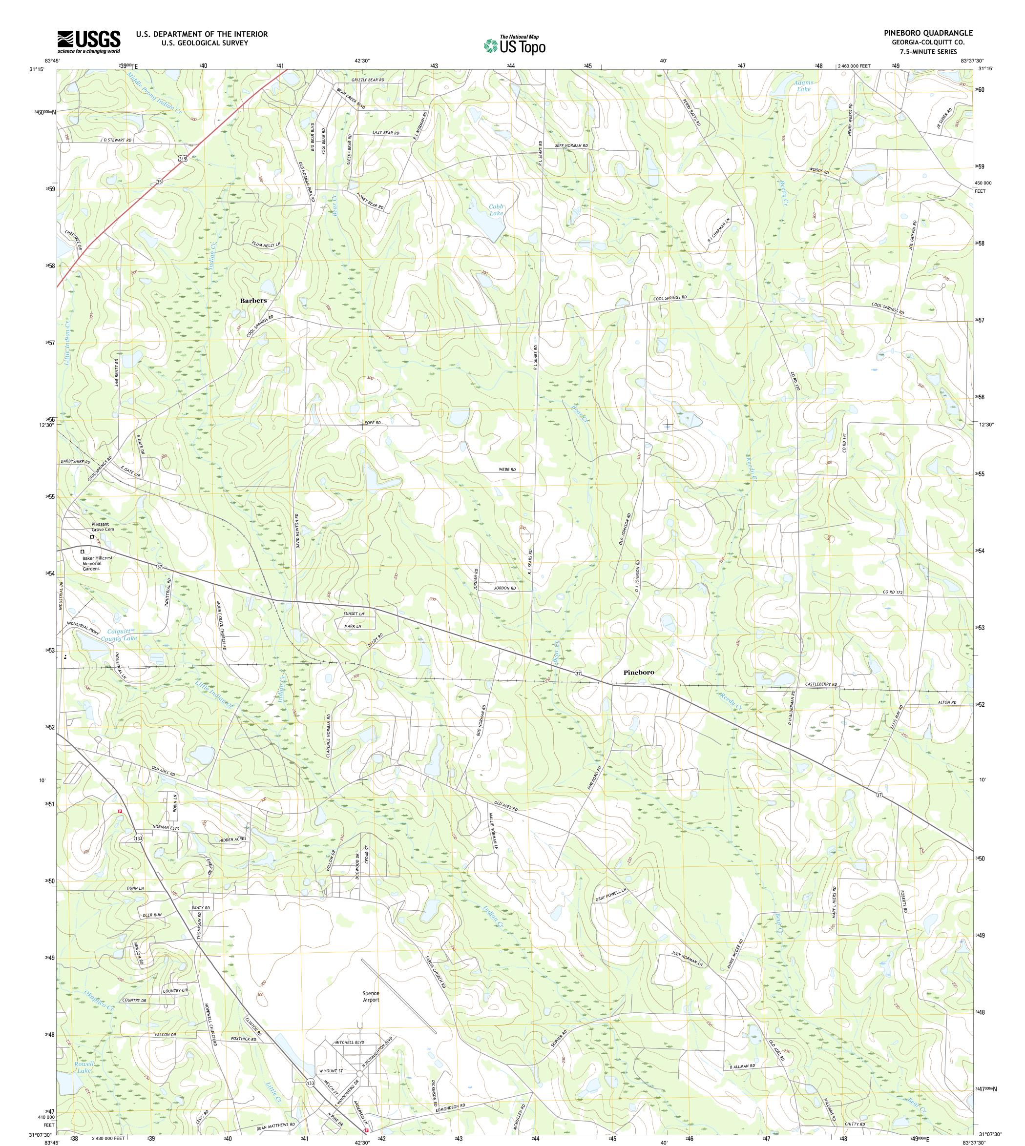
Produced by the United States Geological Survey North American Datum of 1983 (NAD83) World Geodetic System of 1984 (WGS84). Projection and 1 000-meter grid: Universal Transverse Mercator, Zone 17R 10 000-foot ticks: Georgia Coordinate System of 1983 (west zone)
