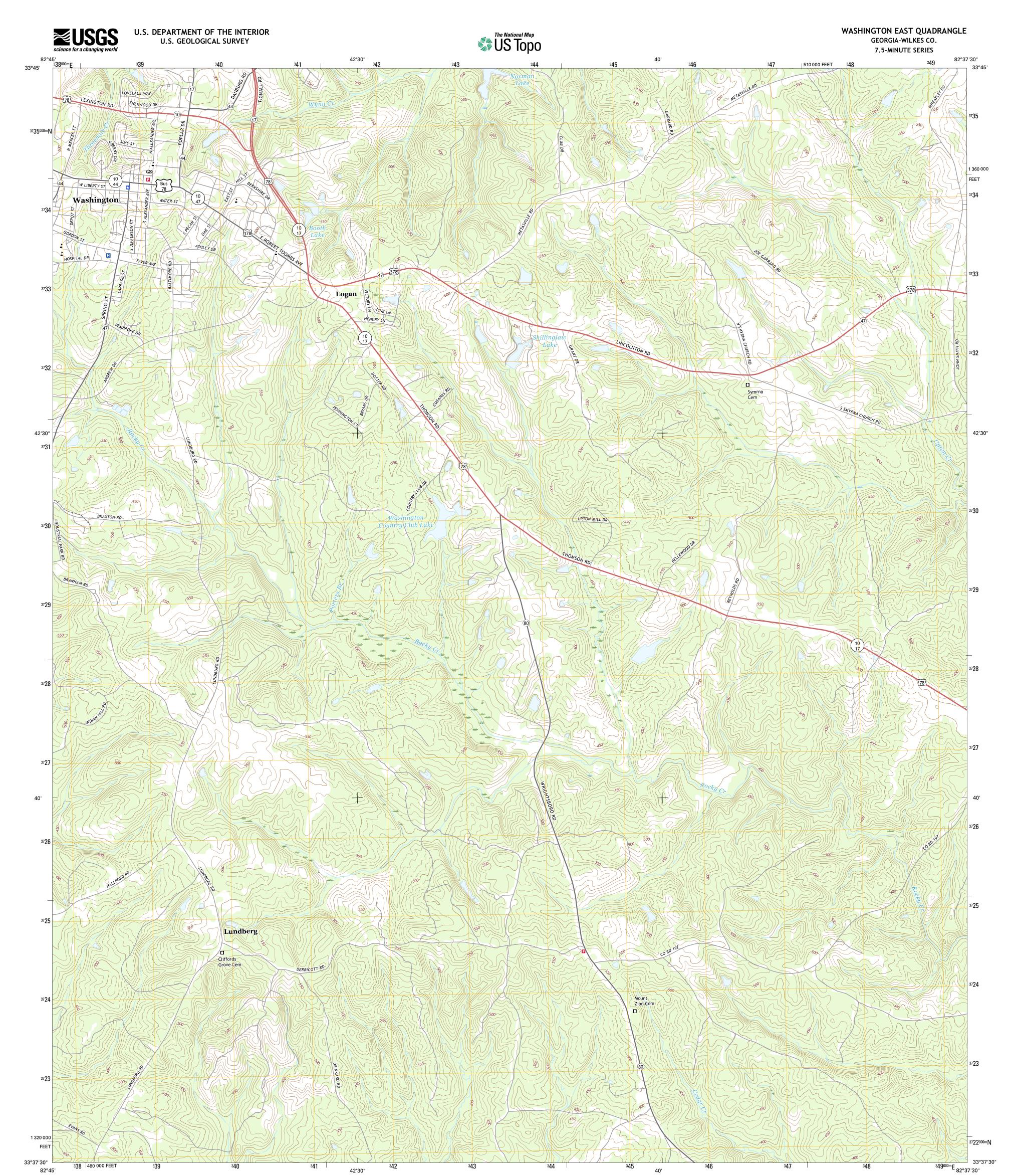
**Produced by the United States Geological Survey** North American Datum of 1983 (NAD83) World Geodetic System of 1984 (WGS84). Projection and 1 000-meter grid: Universal Transverse Mercator, Zone 17S 10 000-foot ticks: Georgia Coordinate System of 1983 (east zone) zone)
