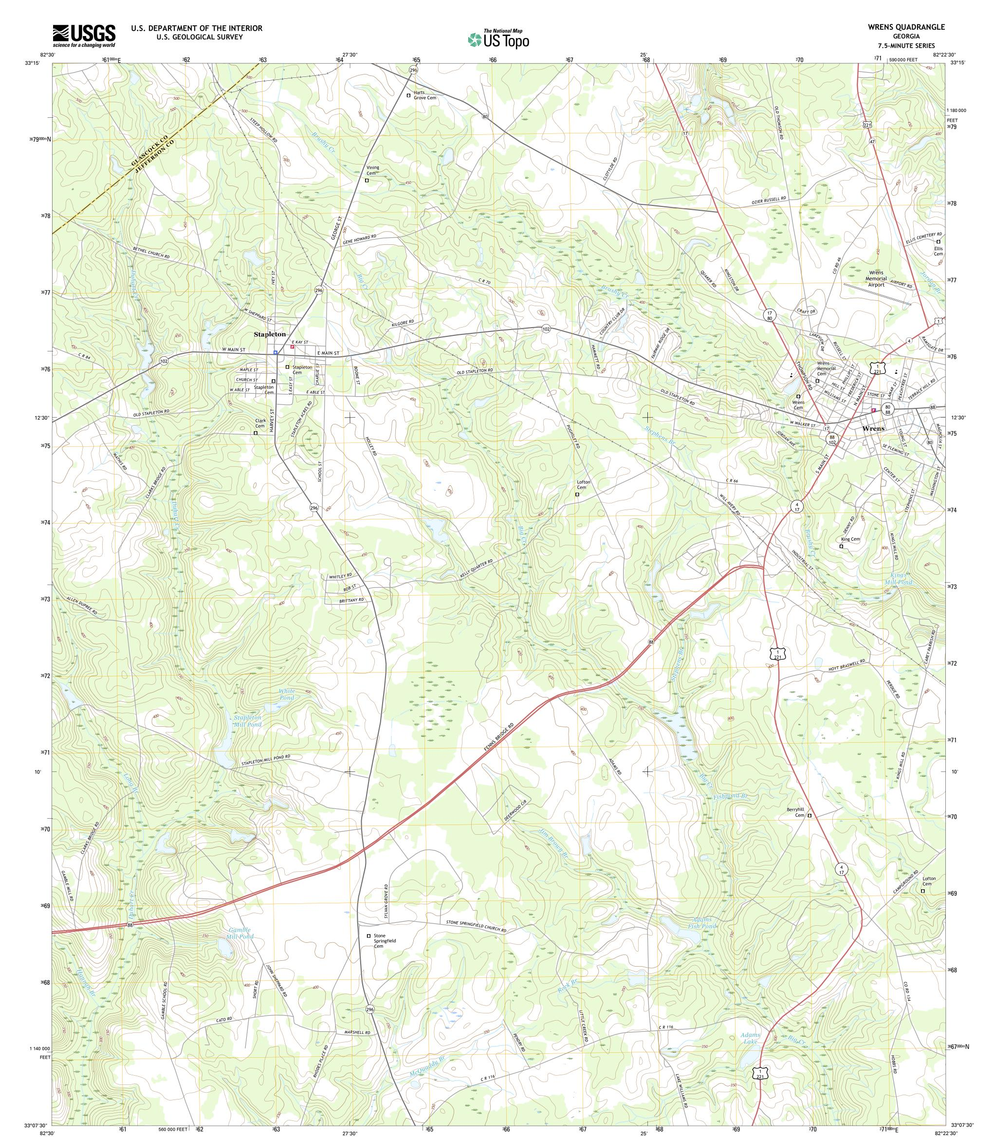
Produced by the United States Geological Survey North American Datum of 1983 (NAD83) World Geodetic System of 1984 (WGS84). Projection and 1 000-meter grid: Universal Transverse Mercator, Zone 17S 10 000-foot ticks: Georgia Coordinate System of 1983 (east zone)
