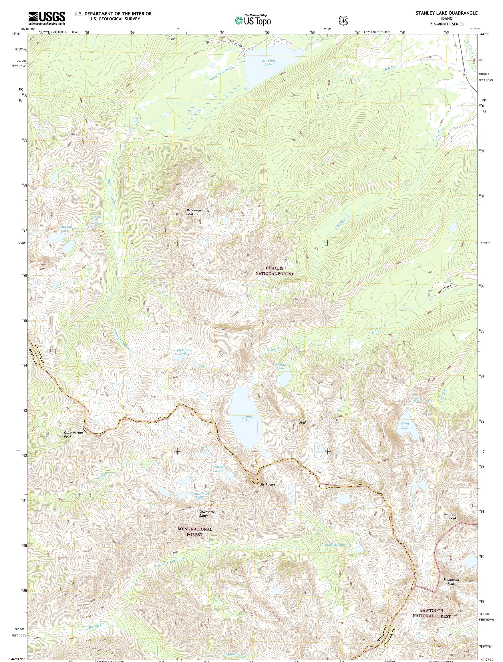
Produced by the United States Geological Survey North American Datum of 1983 (NAD83) World Geodetic System of 1984 (WGS84). Projection and 1 000-meter grid: Universal Transverse Mercator, Zone 11T 10 000-foot ticks: Idaho Coordinate System of 1983 (central and west Zones) west zones)
