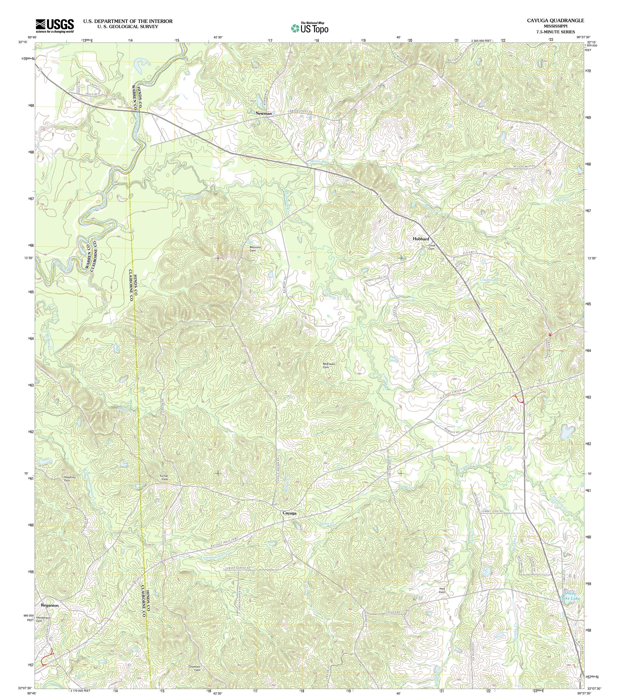
Produced by the United States Geological Survey North American Datum of 1983 (NAD83) World Geodetic System of 1984 (WGS84). Projection and 1 000-meter grid: Universal Transverse Mercator, Zone 15S 10 000-foot ticks: Mississippi Coordinate System of 1983 (west zone)
