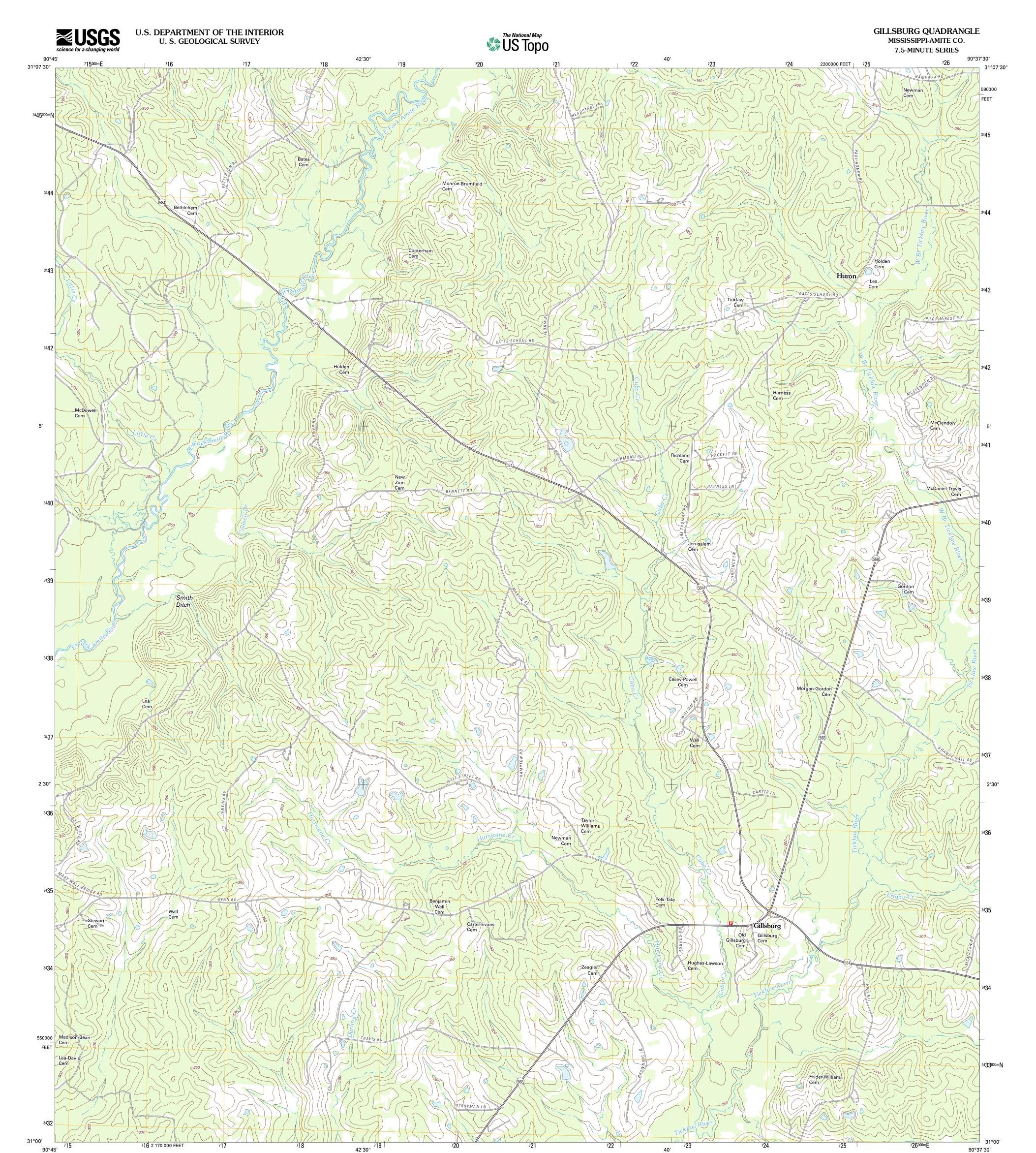
Produced by the United States Geological Survey North American Datum of 1983 (NAD83) World Geodetic System of 1984 (WGS84). Projection and 1 000-meter grid: Universal Transverse Mercator, Zone 15R 10 000-foot ticks: Mississippi Coordinate System of 1983 (west zone)
