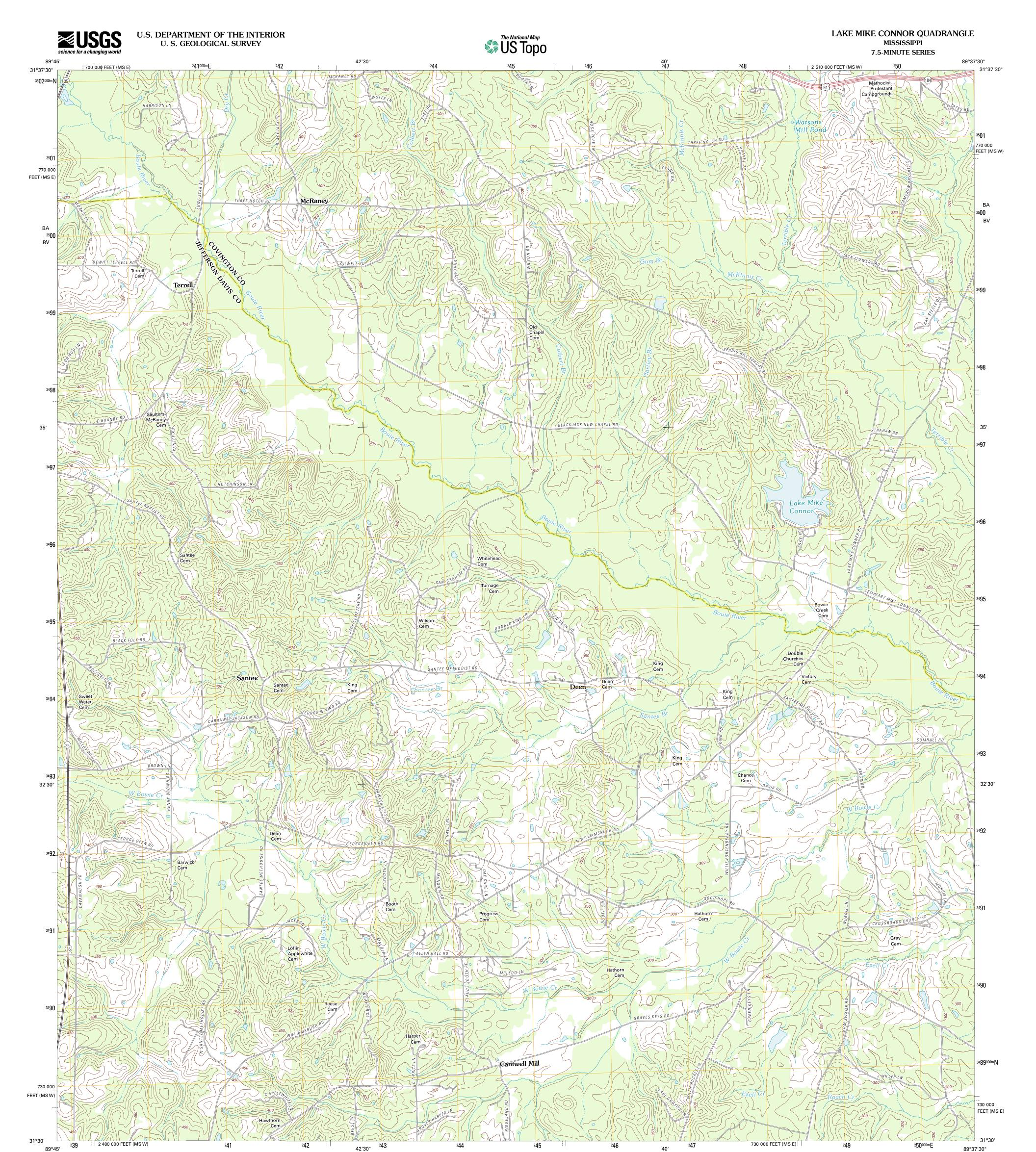
Produced by the United States Geological Survey North American Datum of 1983 (NAD83) World Geodetic System of 1984 (WGS84). Projection and 1 000-meter grid: Universal Transverse Mercator, Zone 16R 10 000-foot ticks: Mississippi Coordinate System of 1983 (west and east zones)
