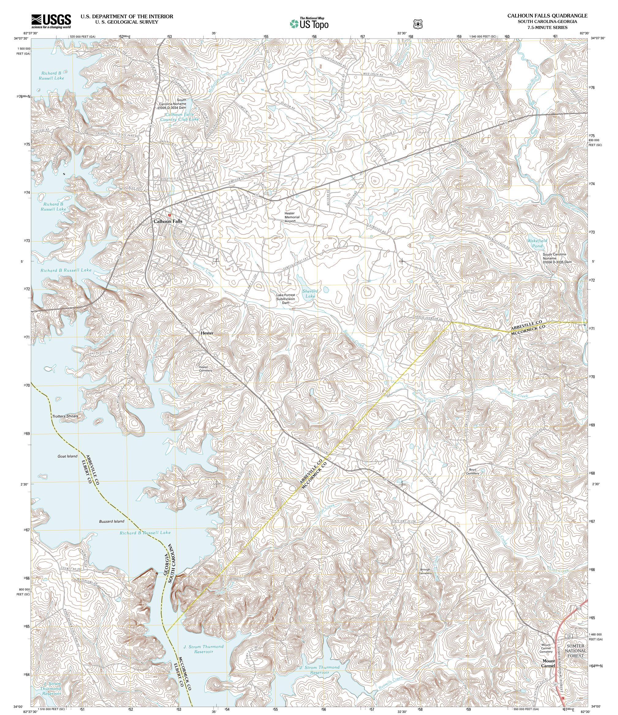
Produced by the United States Geological Survey North American Datum of 1983 (NAD83) World Geodetic System of 1984 (WGS84). Projection and 1 000-meter grid: Universal Transverse Mercator, Zone 17S 10 000-foot ticks: South Carolina Coordinate System of 1983, Georgia Coordinate System of 1983 (east zone)
