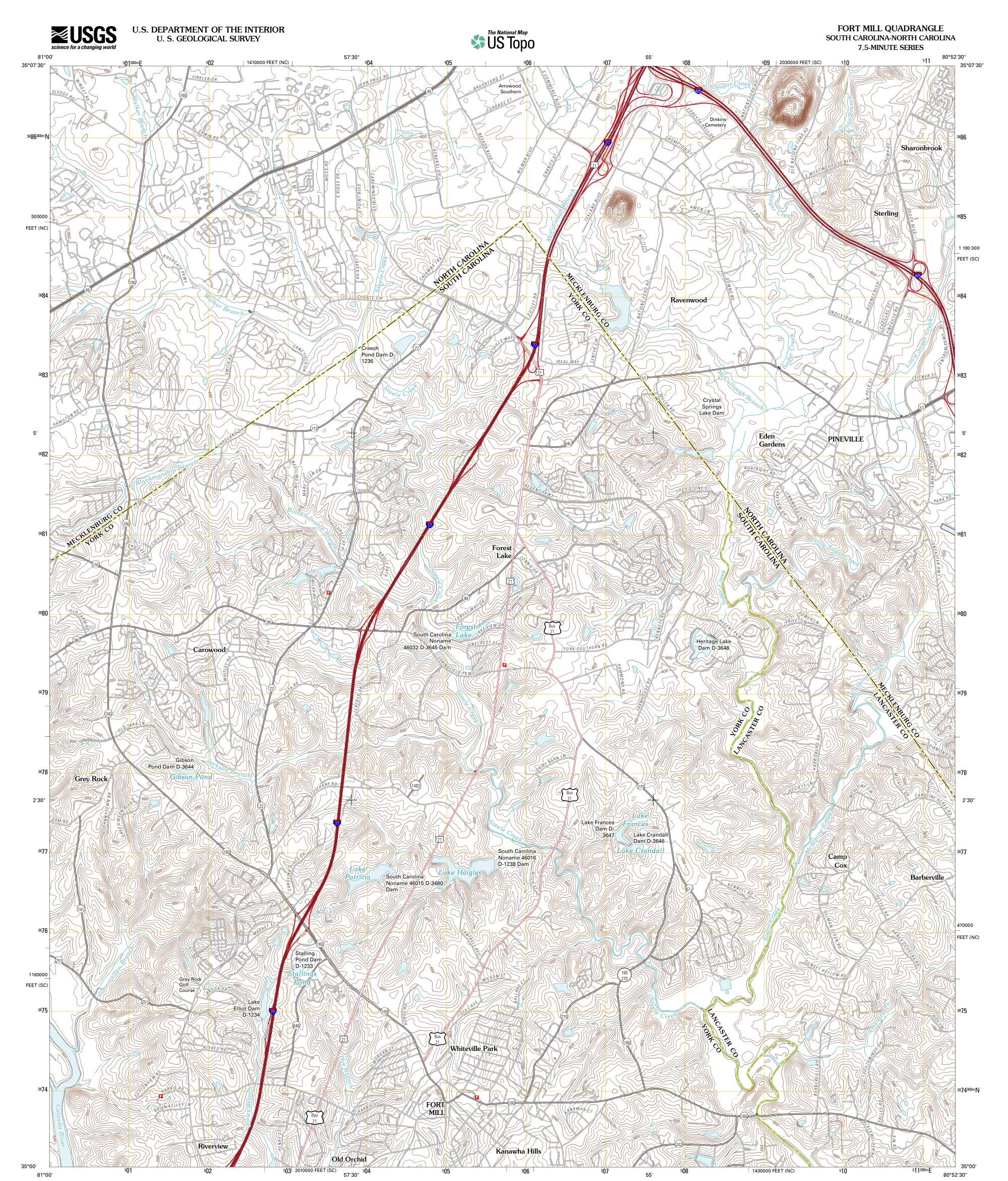
Produced by the United States Geological Survey North American Datum of 1983 (NAD83) World Geodetic System of 1984 (WGS84). Projection and 1 000-meter grid: Universal Transverse Mercator, Zone 17S 10 000-foot ticks: South Carolina Coordinate System of 1983, North Carolina Coordinate System of 1983
