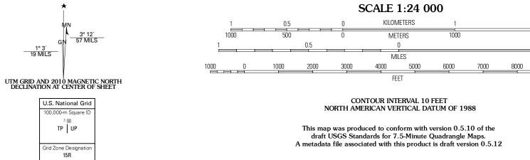
Produced by the United States Geological Survey North American Datum of 1983 (NAD83) World Geodetic System of 1984 (WGS84). Projection and 1 000-meter grid: Universal Transverse Mercator, Zone 15R 10 000-foot ticks: Texas Coordinate System of 1983 (central zone)
