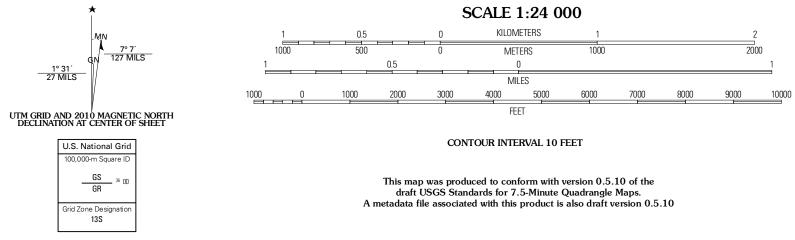
Produced by the United States Geological Survey North American Datum of 1983 (NAD83) World Geodetic System of 1984 (WGS84). Projection and 1 000-meter grid: Universal Transverse Mercator, Zone 13S 10 000-foot ticks: Texas Coordinate System of 1983 (north central zone)
