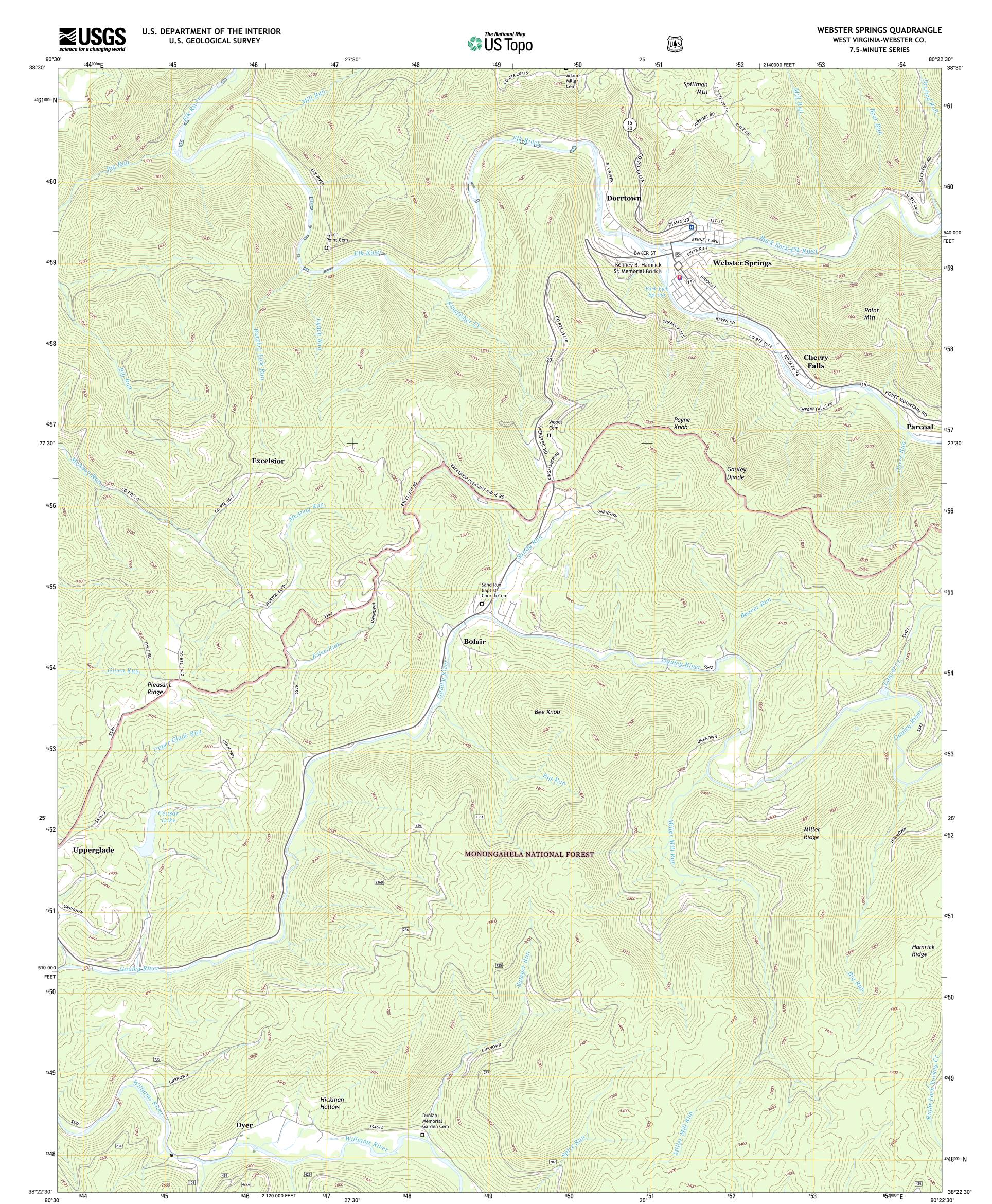
**Produced by the United States Geological Survey** North American Datum of 1983 (NAD83) World Geodetic System of 1984 (WGS84). Projection and 1 000-meter grid: Universal Transverse Mercator, Zone 17S 10 000-foot ticks: West Virginia Coordinate System of 1983 (south zone)
